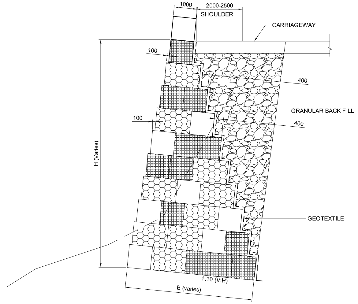
GRAVITY GABION WALL (BACK BATTER) SCALE:-1:100
